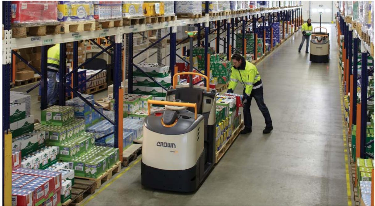
One of the applications that has emerged as a good fit for automation is high-volume picking where the operator is able to remotely advance the forklift, eliminating the need to climb on and off the vehicle multiple times in an aisle.
