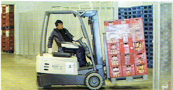
KwaZulu-Natal-based dairy Dairy Day, which produces Honeydew dairy products, has acquired crown equipment from Goscor Lift Truck Company (GLTC) for its 15 000 m 2 processing facility in Howick. Dairy Day acquired six Crown three-wheel electric forklifts with double batteries to cater for double shifts and two Crown powered pallet trucks, also with double batteries
