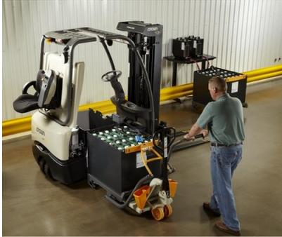
*The fact that the SC 5300 battery can be swapped out quickly [lit. = Through the option of fast swapping the battery] [means] there is no idle time for the forklift truck in three-shift operation*
