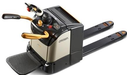
*The WT 3000 has [lit. = offers] suspension that can be adjusted to the operator's bodyweight, hence improved driver comfort*
