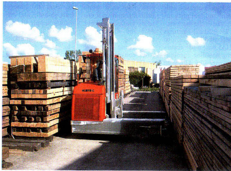
A Hubtex multidirectional and side loader with material for the construction industry.
