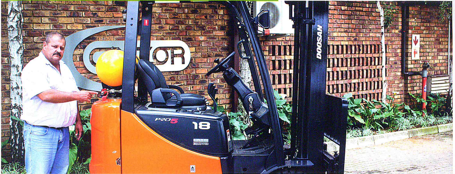
Philip Hoare, national service manager, Goscor Lift Truck Company, showing the quick coupler for CNG refuelling on the specially converted Doosan forklift.
